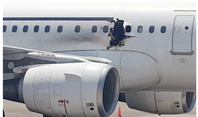
Hole created by a Shabaab suicide bomber onboard Daallo Airlines Flight 159 on February 2, 2016.
